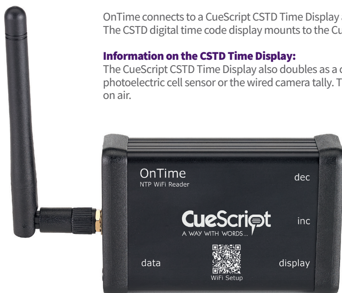
One OnTime unit is required per CSTD Time Display.
